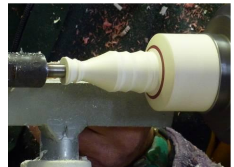
Begin finial shaping by roughing down between centres, retaining mass at headstock
