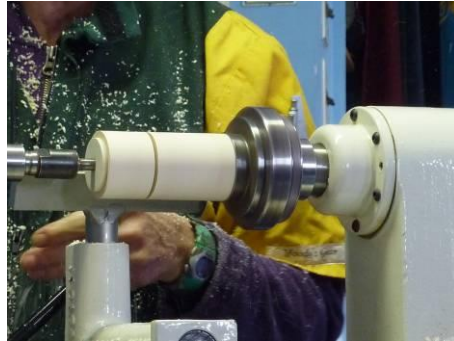
Using a Holly blank it is separated into box and finial
