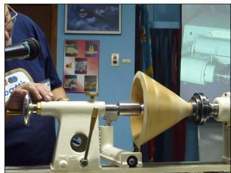
Another way to hold roof – a plug and MT extender.
