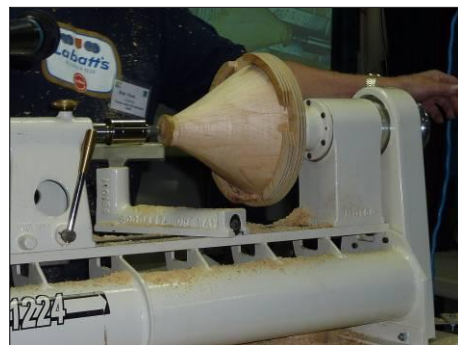
The exterior is held by a jam plate and the tailstock and finish turned.
