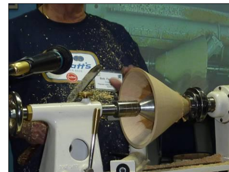
The inside is turned round for an inch or two, where the roof will contact the sides.
