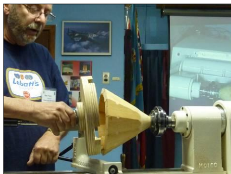
Holding device for truing up roof.
