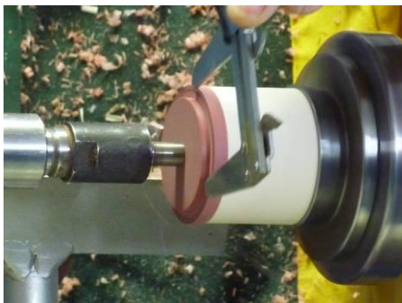
Cut tenon to size, will form contrast ring in box
