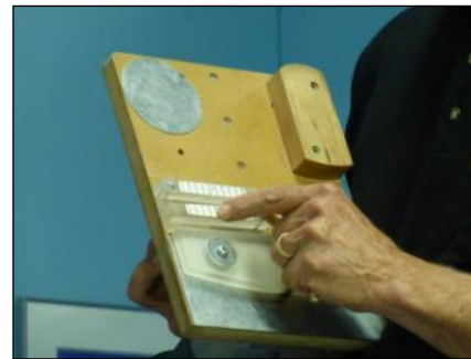
A Jig for sanding the precision flats of his bobbin
