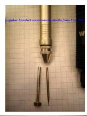
There are carving hand pieces for the Wecheer/Foredom/Dremel tools that convert rotary motion to impact enabling the tools to power carve with chisels such as the "Flexsteel" chisels. Also suitable are the carbide "Kutzall" burrs such as the ball type shown.
