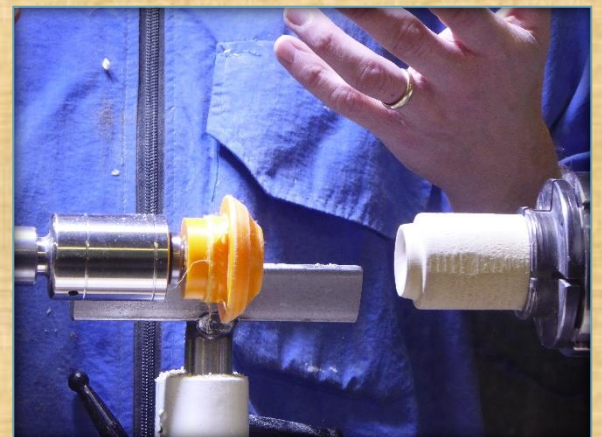
Two examples of cup chucks to hold the sphere for further rounding
