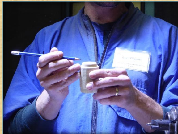
Preparing a cupchuck for later use. The cup will match the template's contour.
