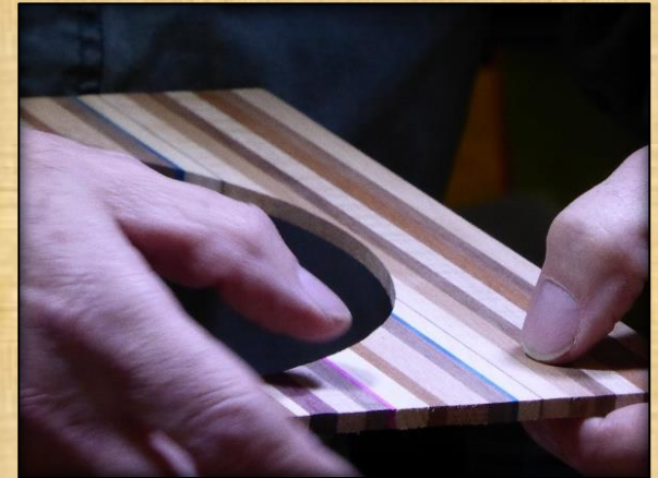
A dizzybowl is essentially a bowl from a board. The "board" is a lamination of different woods set off by veneers to emphasize or highlight the colored slices.
