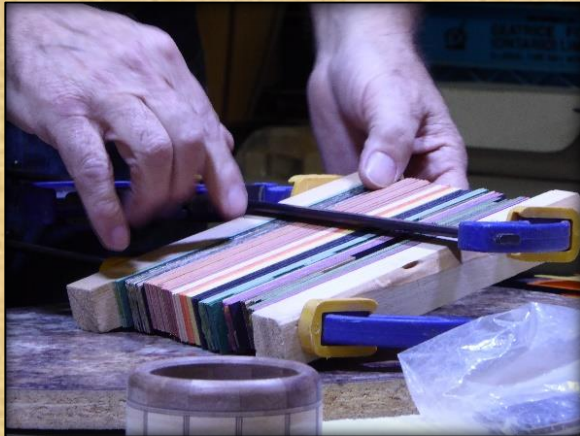
Assembling a laminated board. Carl uses white carpenters glue and ensures complete coverage on both sides of each slice to prevent glue starved joints that could fail
