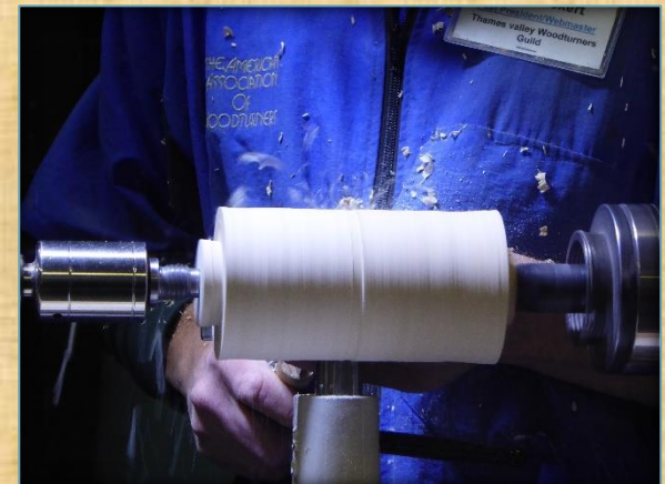
Don't cut any deeper than the design size 2 3/4" dia or your sphere will begin to shrink.
