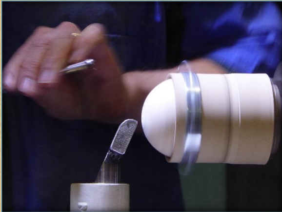
Gently remove wood, use the template frequently and rotate the ball to ensure it maintains it's "round"
