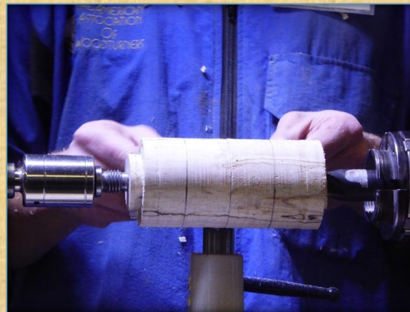
As the diameter approaches our design diameter it is time to mark the boundaries
