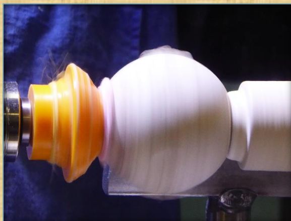
This step is removal of nibs - note "ghost" to be removed
