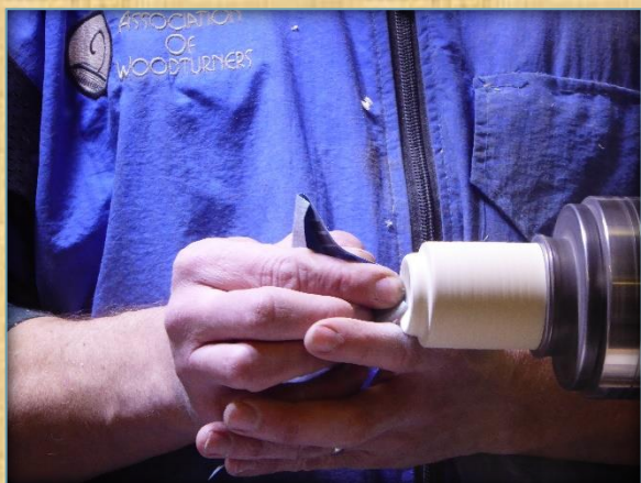
Fine tuning to aid grip and to prevent marring of the sphere
