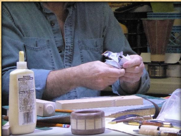
Preparing the lamination, covering both top and bottom to prevent glue adhering to the form.
