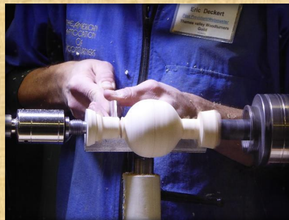
Time to cut sphere free to continue on to the next stage
