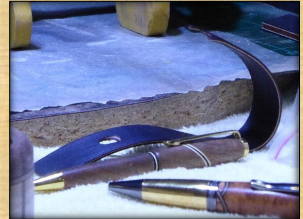
A pen display piece made with a simple form from bending veneers around a form (3 layer laminate).
